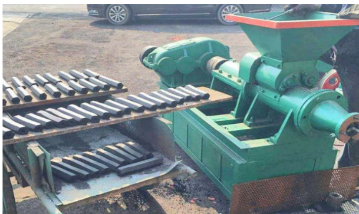
Figure 2.4: Screw Extrusion briquetting machine (making cylindrical briquettes)
