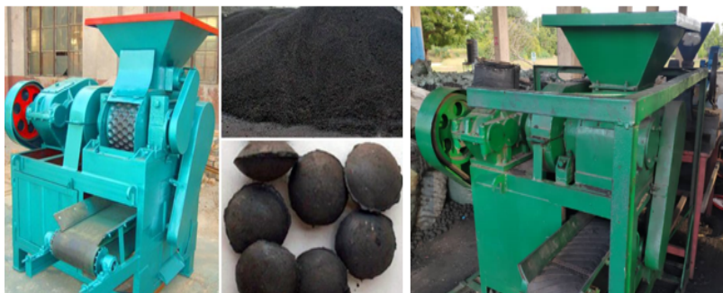
Figure 2.5: Roller press briquetting machine (making oval briquettes)
