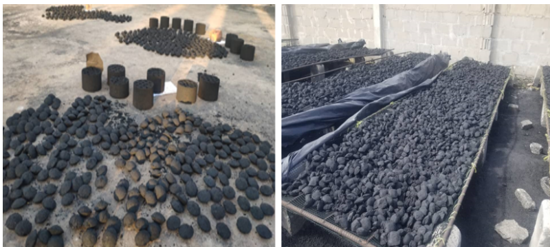
Figure 2.8: Sun drying of biomass briquette
