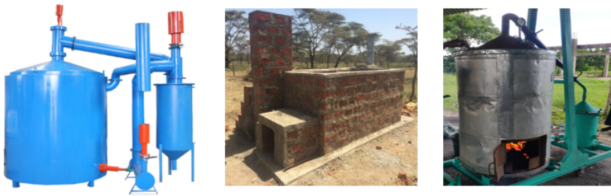
Figure 3.7: Different types of Carbonizer machines
