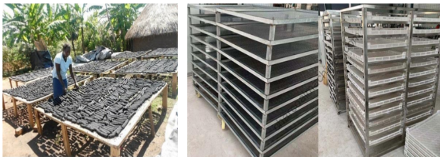
Figure 3.2. The sun/open air-drying facilities for biomass briquettes
