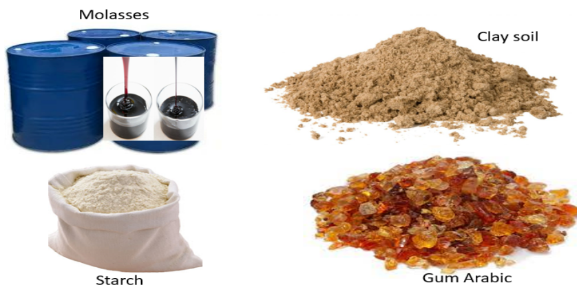
Figure 2.3: The common types of binder used in production of biomass briquettes.
